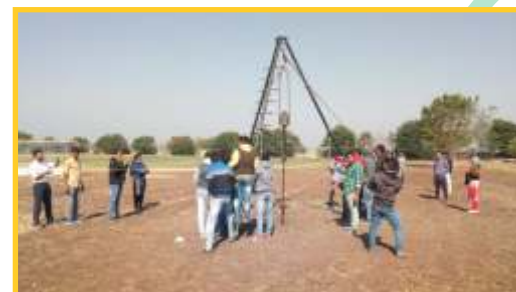
"The Assembly is fitted exactly and ready to driven for safe collection of undisturbed sample under observation of Prof. Vimal Patel, Prof. Natasha Sagar and Prof. Kajal Dudhatra"
